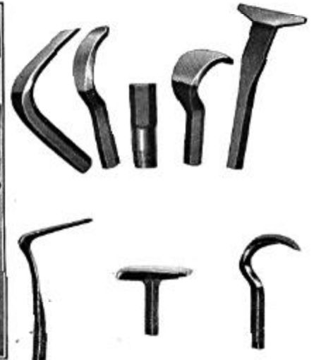
Body Jack Soons that work behind inner panel constructions at all points of the body, with working faces that conform to any damaged area. This avoids localized pressure and distortion.
