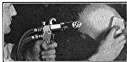
PADDLE SOLDERING —After spraying sufficient solder the bowl is again turned from the flame and the operator then uses the gun to heat the solder to plastic form for moulding as desired. This is necessary in all cases of solder spraying to obtain uniform texture free from air holes and flaws.
