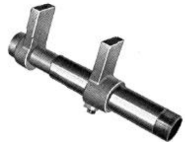
Wide Range Spreading and Clamping Unit. From a short coupled spreading range of 2"—19" to a wide clamping range, when mounted on opposite ends of Jack Unit, that will take a cross section of the body.
