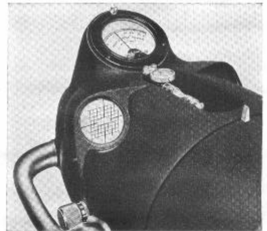
5. The internal screen shows the pattern of the beam against a graduated cross-grid ruling, and enables the customer to see the setting of his lights.
