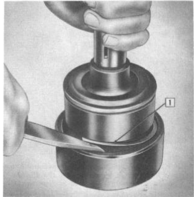
FIGURE 19—Remove the Snap Ring to Separate the Ring Gear From the Main Shaft
