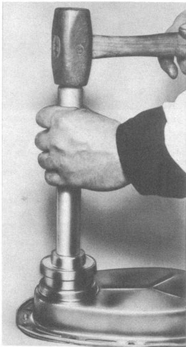
FIGURE 16—Removing Timing Chain Cover Oil Seal—"Hornet" and "Wasp" Series
