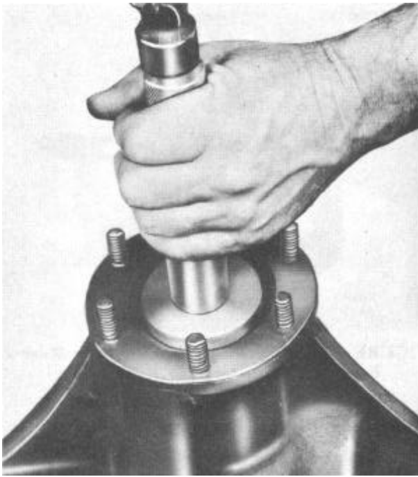
FIGURE 24—Installing Front Pinion Bearing Cup
