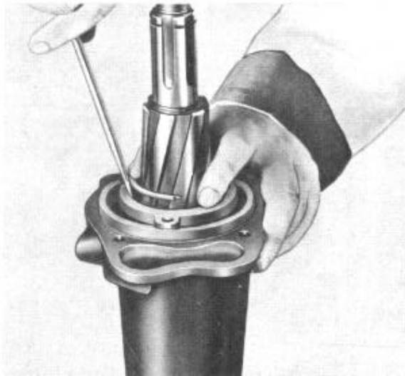
FIGURE 11—Remove the Snap Ring From the Front of the Rear Bearing Cap
