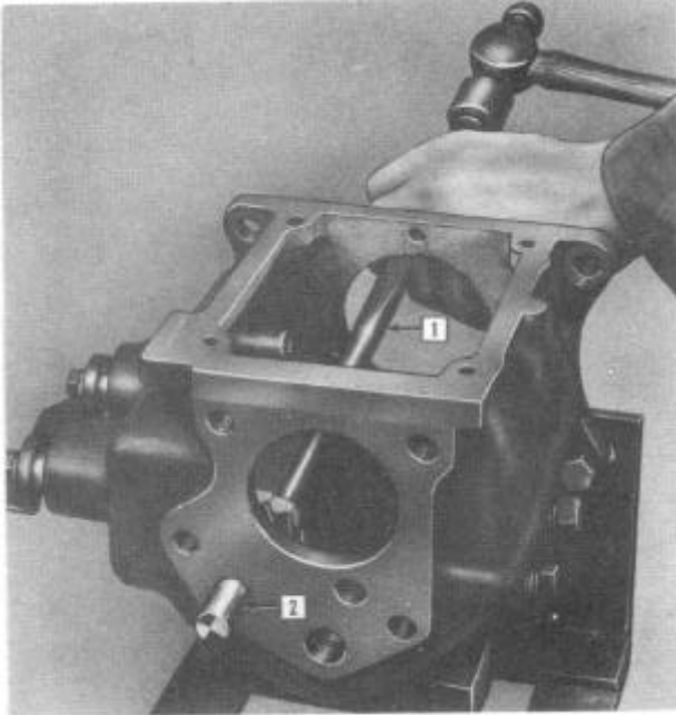
FIGURE 43—To Remove the Reverse Idler Gear Shaft, Drive it Out the Rear of the Case With a Brass Drift
