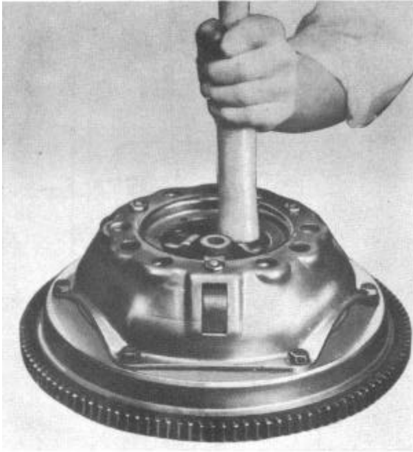
FIGURE 8—Each Lever Should be Depressed Several Times to Settle all Parts in Their Proper Positions
