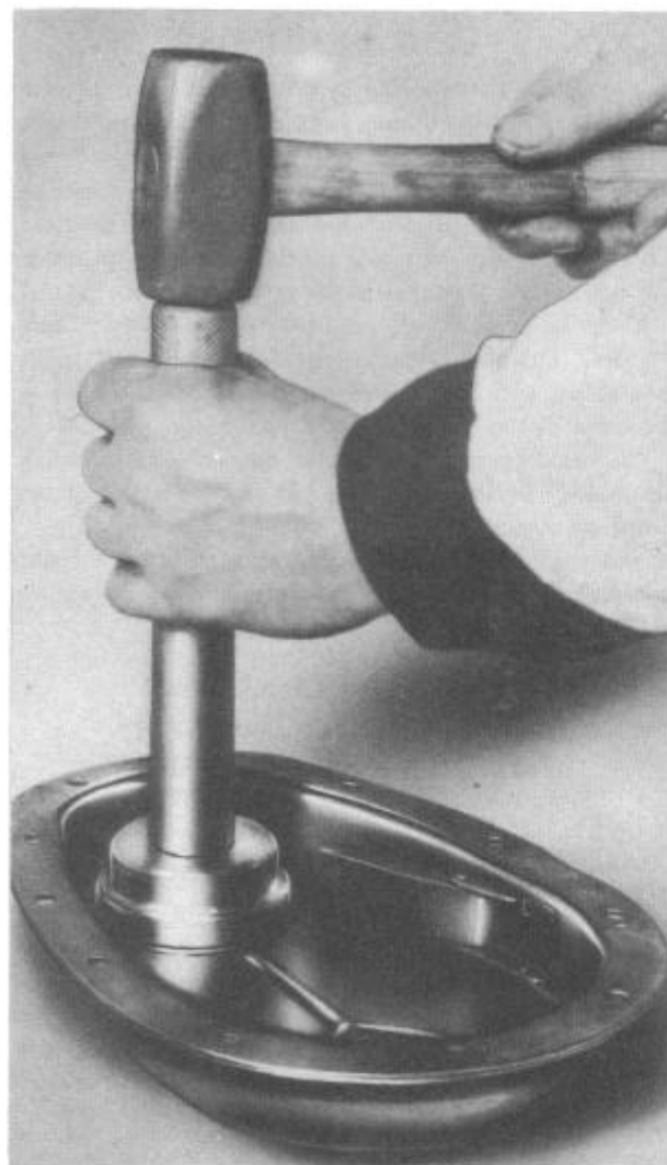
FIGURE 17—Installing Timing Chain Cover Oil Seal—"Hornet" and "Wasp" Series
