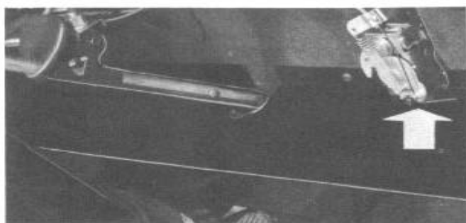
FIGURE 8—Water Control Valve Capillary Tube Location—"Hornet" and "Wasp" Series
