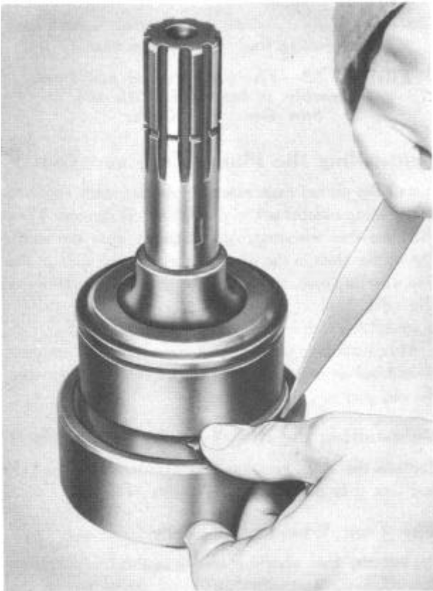
FIGURE 34—Install a Snap Ring to Hold the Ring Gear on the Main Shaft
