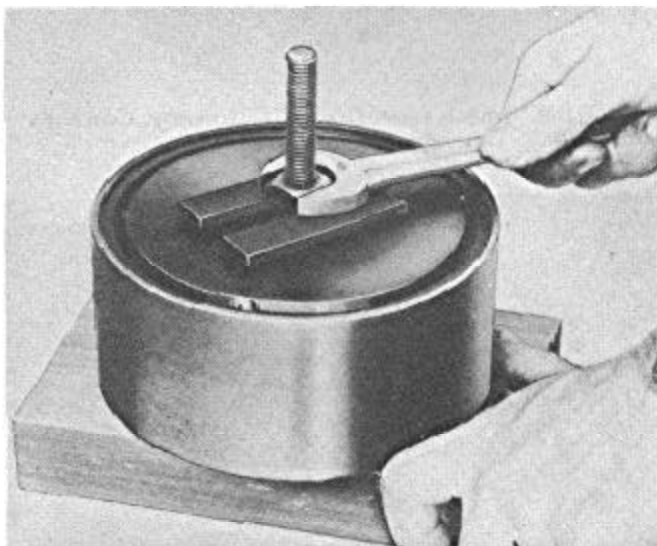
FIGURE 151—Compressing Clutch Drum.
