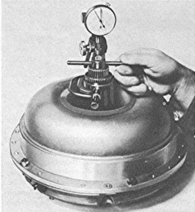
FIGURE 35—Measure Reactor Shaft End Play
