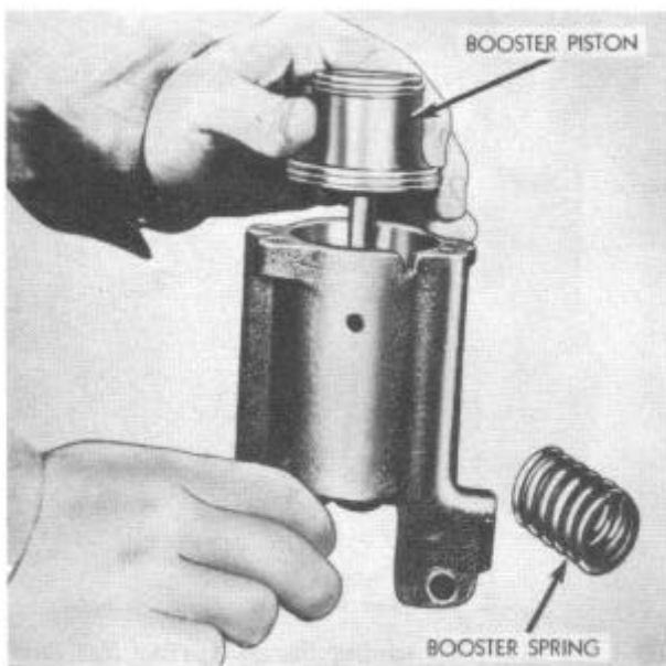
FIGURE 57—Removing Booster Piston
