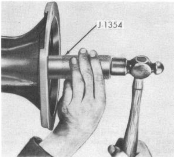
FIGURE 46—Installing Rear Bearing Retainer Oil Seal
