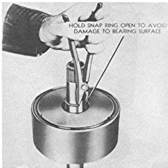
FIGURE 150—Removing Snap Ring from Recess in Front Unit
