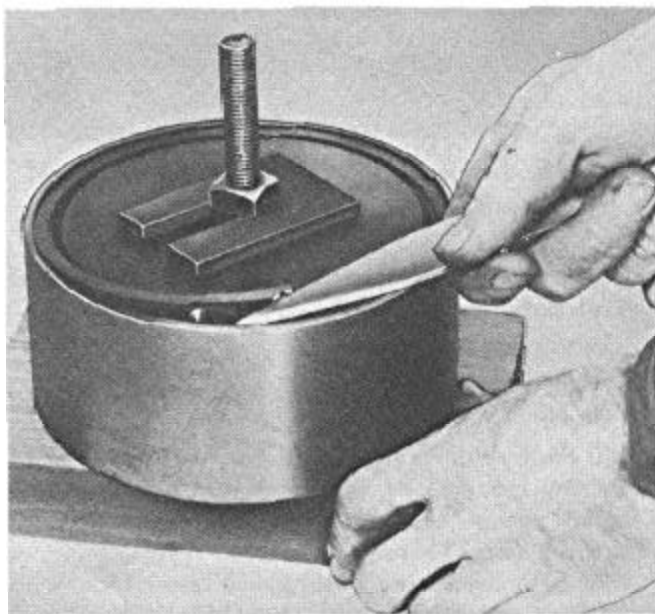
FIGURE 152—Removing Clutch Drum Snap Ring
