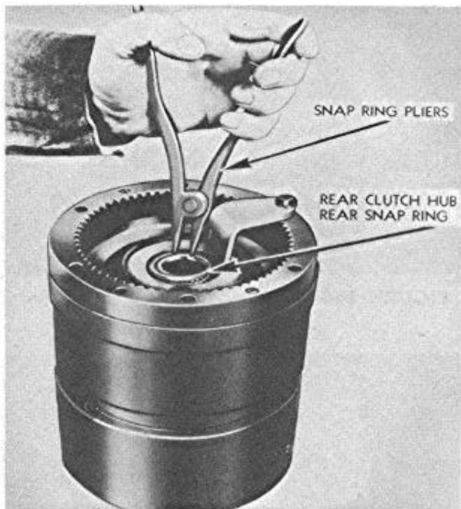
FIGURE 149—Removing Rear Clutch Hub Rear Snap Ring
