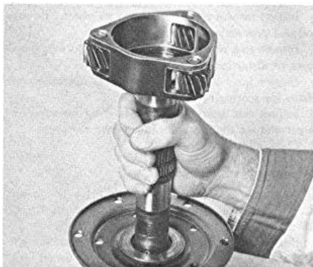
FIGURE 136—Installing Reverse Center Gear on Output Shaft
