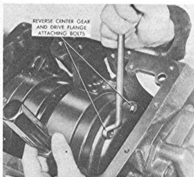
FIGURE 129—Removing Reverse Center Gear and Drive Flange Attaching Bolts
