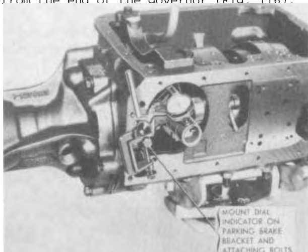
FIGURE 116—Checking Governor Runout
