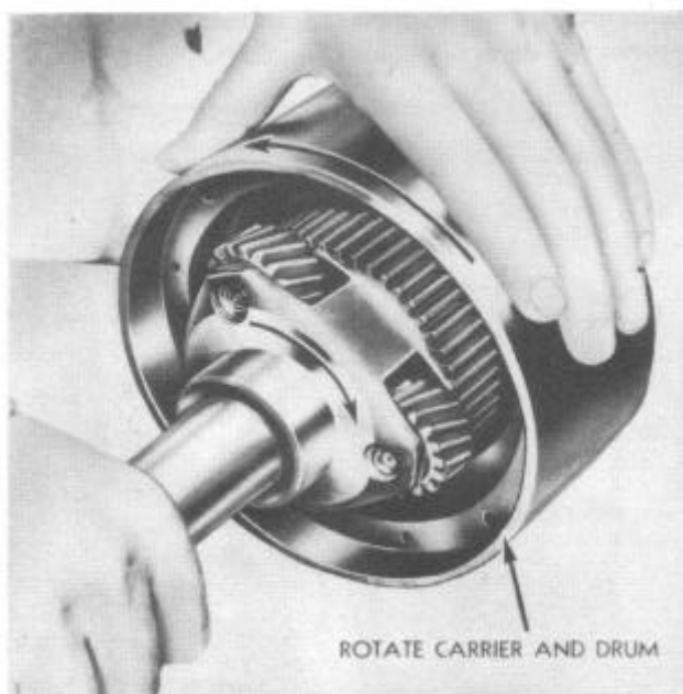
FIGURE 166—Aligning Clutch Plates
