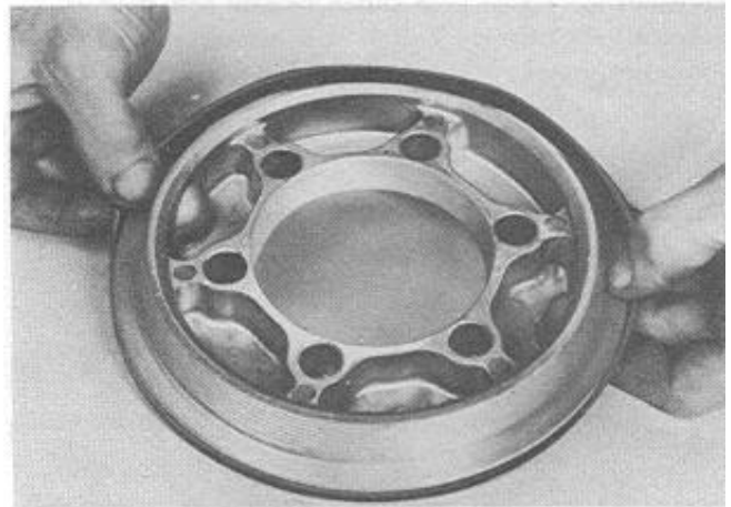
FIGURE 140—Installing Reverse Cone Piston Outer Seal
