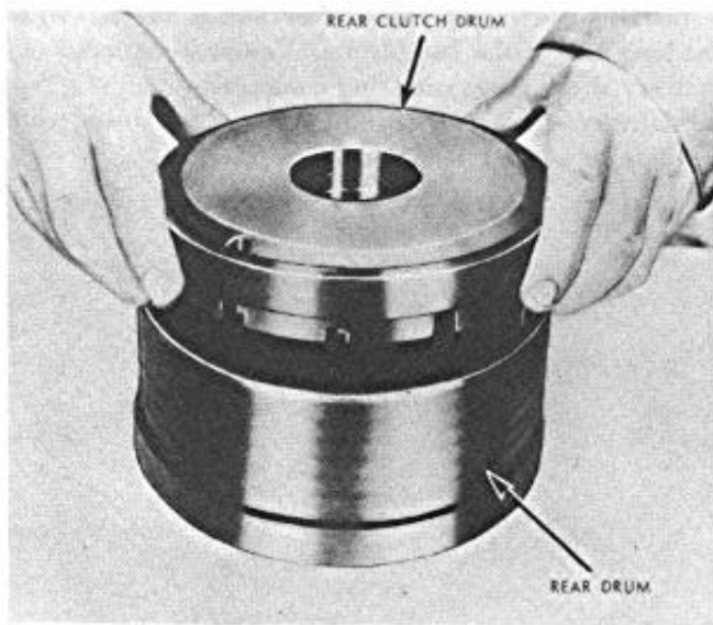
FIGURE 175—Installing Rear Clutch Drum
