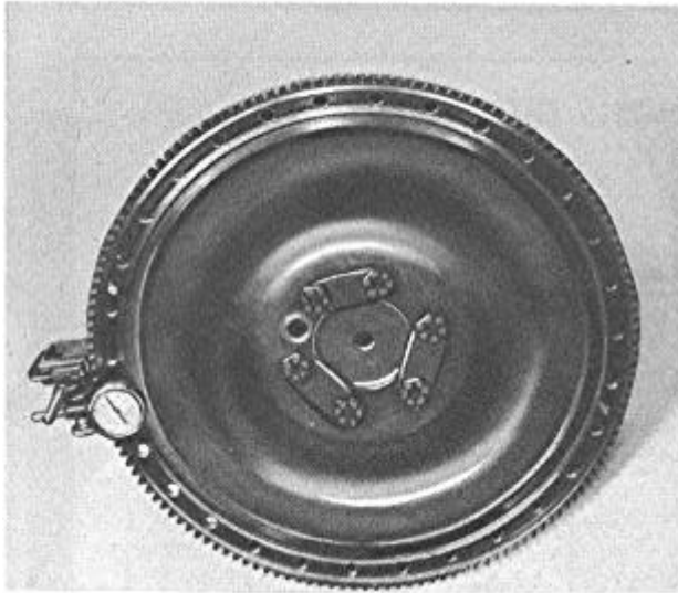
FIGURE 214—Checking Flywheel Runout
