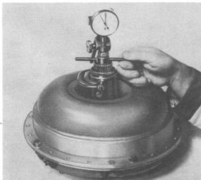
FIGURE 61—Check the Reactor Shaft End Play
