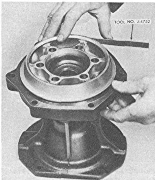
FIGURE 141—Installing Reverse Cone Piston in Rear Bearing Retainer
