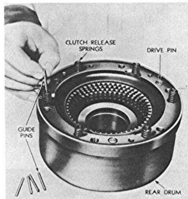
FIGURE 177—Installing Clutch Release Springs and Guide Pins
