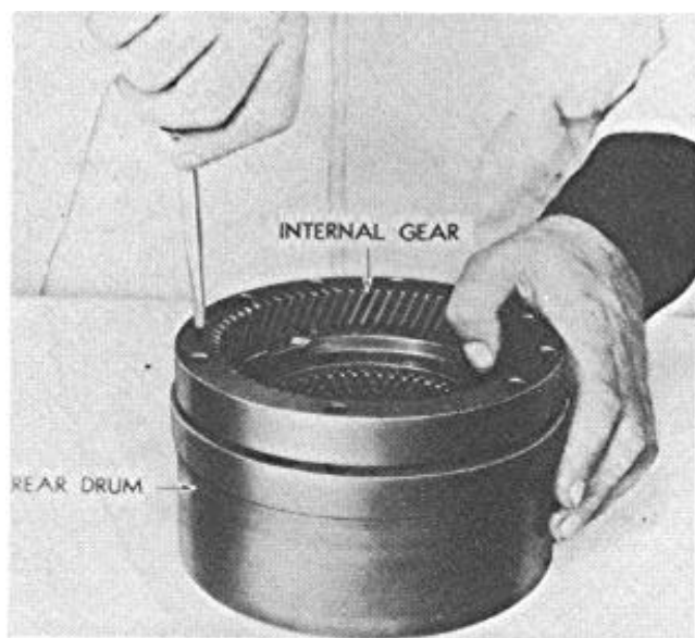
FIGURE 178—Assembling Internal Gear to Rear Drum
