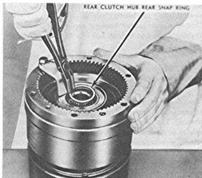
FIGURE 183—Installing Rear Clutch Hub Rear Snap Ring
