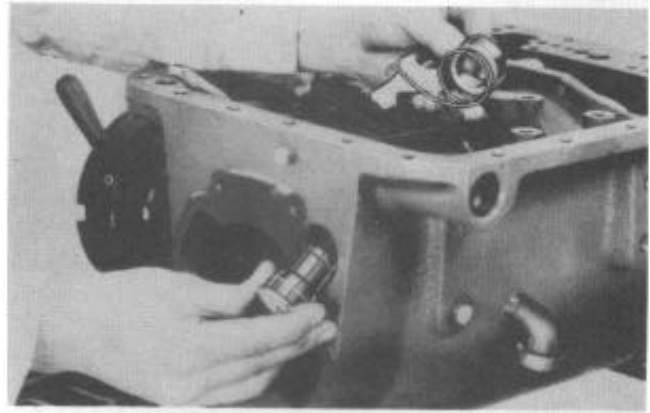
FIGURE 32—Removing the Parking Lock Support, Lever and Spring
