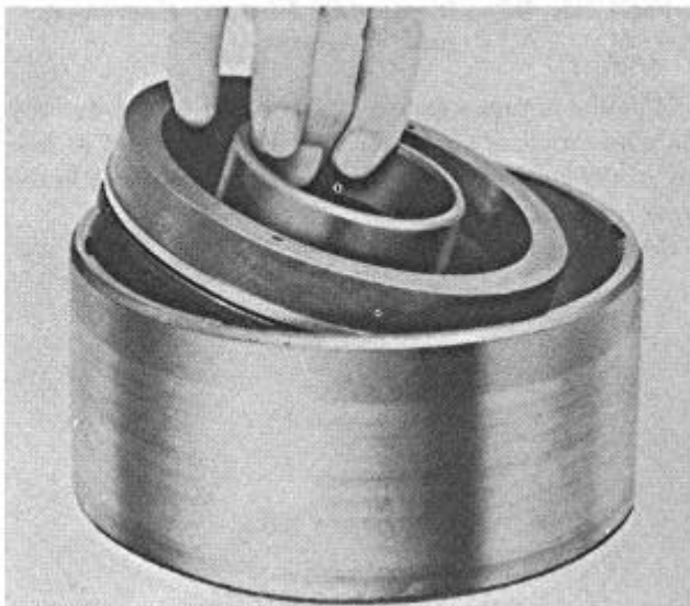
FIGURE 91—Place the Piston in the Housing
