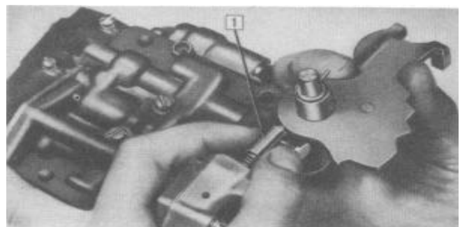
FIGURE 95—Installing Detent Plunger Retainer
