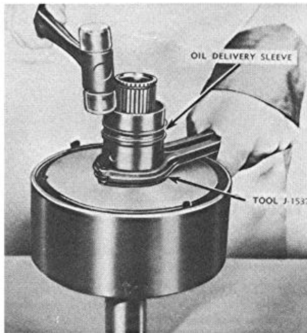
FIGURE 182—Installing Oil Delivery Sleeve
