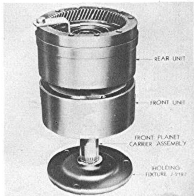
FIGURE 148—Disassembly of Front and Rear Units
