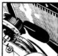
Ignition Timing Breaker Points to Open: 5° B.T.D.C.
