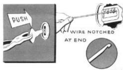
DON'T BE SHUT OUT -- If key breaks in locked car door, hold the stub firmly (preferably with pliers), push it into slot as far as it will go and, maintaining steady inward pressure, you may be able to turn key SLOWLY. Later, in the comfort of your garage, you can try fishing out the broken part with a piece of fine piano wire filed into a "fish-hook barb" at the end.
