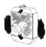
RADIATOR TEST — When you clean your cooling system here's how to tell if the radiator is clogged (provided bottom outlet bends upward): Drain system, disconnect hoses, and plug radiator openings with stoppers. Fill radiator, leaving cap off. Now pull bottom plug. Water should spout several inches high (see sketch). Otherwise, the radiator needs to be washed out with garden hose, cleaned with Hudson Radiator Flush, or pressure-flushed by your Hudson dealer.
