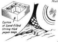
PAPER-BAG SAND "BOMBS" — To free your car when stuck in ice or snow, carry a carton containing a few small paper bags packed with sand, ashes or gravel and tied with string. Handy, they take little room and make no mess . . . yet one tossed under a helplessly spinning wheel usually provides plenty of traction.
