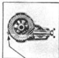
10,000 MILES DIFFERENTIAL ** CHECK LEVEL FREQUENTLY USE S.A.E. 90 MULTI-PURPOSE GEAR LUBRICANT
