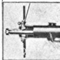
10,000 MILES REAR WHEEL BEARINGS CAPACITY 1½ OUNCES 2 POINTS USE MILLED SODIUM SOIAP BASE GREASE
