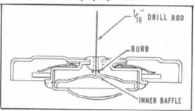
Should any of these Gas Filler Caps that are not properly vented be found in the field, either on cars or in stock, the vent can be opened by inserting a  $\frac{1}{16}$ " drill rod through the vent hole in rivet until the end contacts the inner baffle then tap it sufficient to force the baffle down  $\frac{1}{8}$ " as shown in the illustration.
