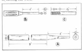
"A" is used for aligning the countershaft gear and thrust washers with the openings in the standard transmission case preliminary to installing the countershaft. This tool may be made up of a straight grain hardwood and of the dimensions shown in sketch.
