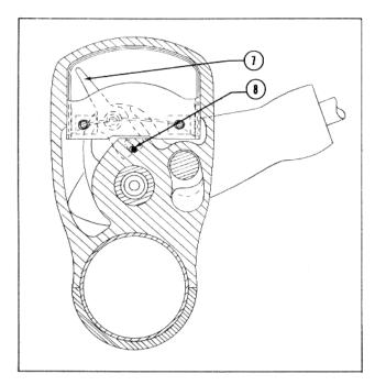
Using a small  $\frac{3}{32}$ " punch, knock-out drive indicator pin (5) which retains drive indicator (7) and drive indicator spring washer (6) to shift control tube.
