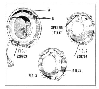
Mounting Ring, #220704, Figure #2 is currently used on all Models from 1950 and uses a single retaining spring, retained by Clip "A" in the Headlamp Housing Figure #1.
