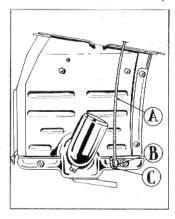
The capillary tube clip "B" Part number 301-889, is mounted facing the front of the heater and the end of the capillary tube is inserted through the clip and bent back 180° to secure the tube to the clip as shown at "C".
