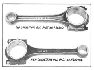
Due to the difference in weight, Connecting Rods of one type MUST NOT be installed in an Engine having Rods of the other type—only as a complete set are they interchangeable. The only positive way to distinguish the two Rods is by the forging numbers on the "I" Beam Section, as shown above.
