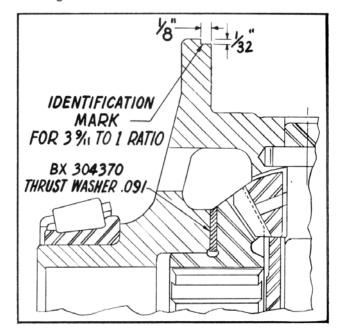
These Differential Cases in both production and service are marked with a yellow paint band at the junction of the right and left halves. This new case that may be used with the 3-9/11 to 1 axle ratio will bear the identification mark as outlined on page 86 of the May Service Merchandiser and as shown in the illustration above.
