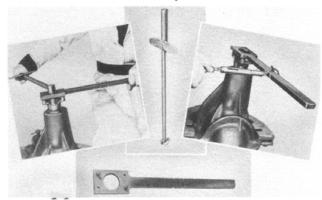
Illustrated above is a special tool that enables the mechanic to hold the companion flange of the transmission or rear axle while tightening the holding nut to an exact torque. The tool provides sufficient leverage for one man to do this work rapidly yet accurately. The rear axle companion flange nut is tightened to 200 ft. lbs. using torque wrench J 1264, as shown in Figure 1.
