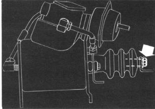
It is important that this cap screw be kept tight. Erratic shifting and gear clashing will result, should this cap screw become loose.
