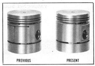
It will be noted in the illustration above that the new or present type Piston has no "T" slot and has a relief at each Piston Pin boss opening. The internal ribbing and smoke holes have been changed. The new Piston has the number 304503 cast on the inner wall. Do not order by this number.
