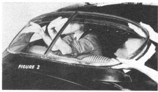
Remove broken glass fragments and all of the old sealer from the rear window recess in the car body also from the window retainer weatherstrip recess. Remove window glass reveal mouldings from weatherstrip also the center bar reveal moulding by prying it loose from center bar. Loosen the five retaining screws in the center bar moulding and window glass retainer to allow for removal and installation of the new glass.
