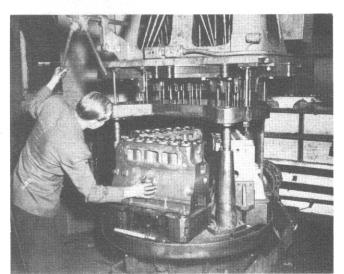
For speed and accuracy, a multiple drill ... drills the twenty-seven (27) cylinder head stud holes ... thereby guaranteeing true alignment when installing cylinder head and gasket.
