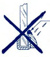
PAST METHOD OF ATTEMPTING TO SEAL BY AN OVERLAY WHICH BECAUSE OF VIBRATION AND SHRINKAGE WILL LEAVE THE GLASS AND EXPOSE THE AREA THAT LEAKS
