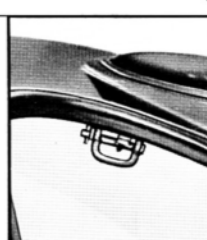
REAR COMPARTMENT DOOR STRIKER ENGINE OIL ON STRIKER HINGE PIN AND SPRING. 2 POINTS EACH SIDE.
