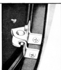
REAR COMPARTMENT DOOR LATCH CLAMPING LEVER WATER RESISTANT GREASE ON CLAMPING LEVER, ENGINE OIL ON LATCH LINK AND PIVOT PIN. 3 POINTS EACH SIDE.
