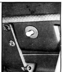
COURTESY LIGHT SWITCH WATER RESISTANT GREASE ON SWITCH PLUNGER. 1 POINT EACH DOOR.
