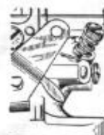
Idle Adjustment Screw Setting 1/4 to 2/4 Turns Open
