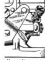
Idle Adjustment Screw Setting 1/2 to 1 1/2 Turns Open
