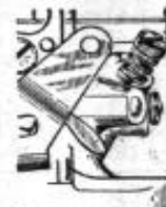
Idle Adjustment Screw Setting ¾ to 1¾ Turns Open
