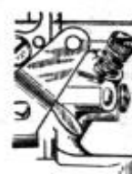
Idle Adjustment Screw Setting 1/2 to 1 1/2 Turns Open
