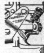
Idle Adjustment Screw Setting 3/4 to 1 3/4 Turns Open
