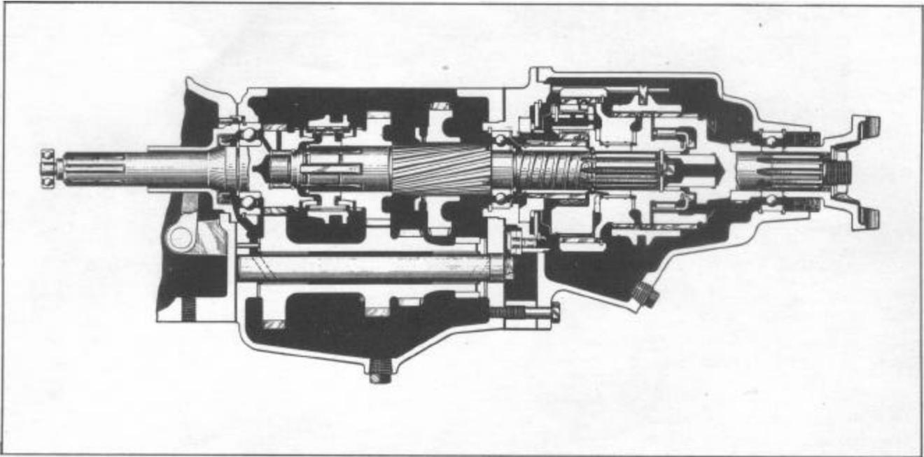
lined bushings operating on a stationary countershaft. Bronze and steel washers located at both ends of the countershaft absorb end thrust. The reverse idler gear is also fitted with a bushing which operates on the stationary reverse idler gear shaft.
