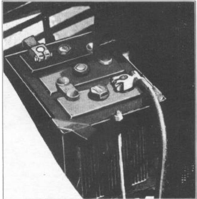
The battery used in six cylinder models has a rating of 96 ampere hours while the one used on eight cylinder models is rated at 108 ampere hours. The S.A.E. classification is 1-ME for the six cylinder battery and 2-ME for the eight cylinder battery.
