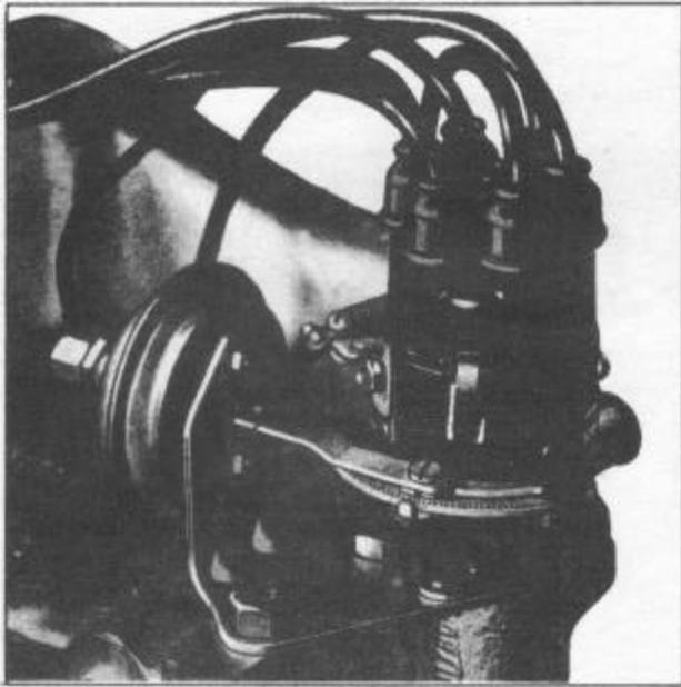
the engine while the eight cylinder distributor is mounted on the side of the crankcase and is driven directly by the camshaft.
