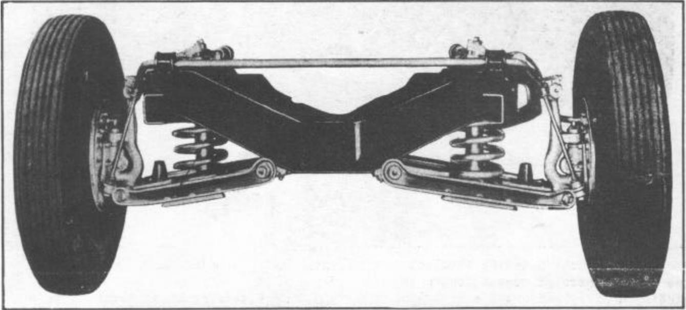
The upper and lower suspension arm and spindle support assemblies are mounted in threaded bushings adjustable for wear and fitted with rubber sleeves for protection against dirt and water. Attachment of the top of the steering spindle support to the upper suspension arm on each side is made through threaded eccentric bushings which also provide the necessary adjustment to obtain the correct caster and camber settings.
