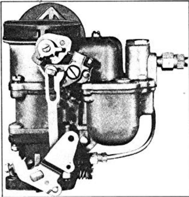
anti-percolating valve to reduce vapor pressure and the possibility of vapor lock. Heat deflecting shields and special thick insulating gaskets are used between the carburetor and manifold to reduce the heat transferred to the carburetor.
