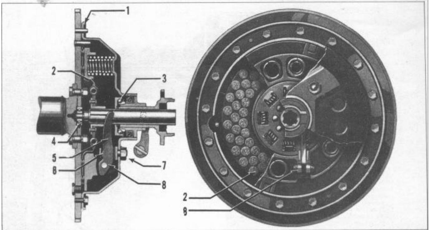
insures smooth starting and long life for all working parts. The driving plate of the 9 inch clutch contains 90 cork inserts; the ten inch plate has 108 corks and the light weight of this part greatly assists gear shifting by reducing the tendency to spin.
