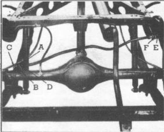
frame member on the right side. The latter part has been redesigned and reinforced and is now attached to the frame side member by riveting and welding providing a much stronger anchorage than heretofore. frame member on the right side. The latter part has been redesigned and reinforced and is now attached to the frame side member by riveting and welding providing a much stronger anchorage than heretofore
