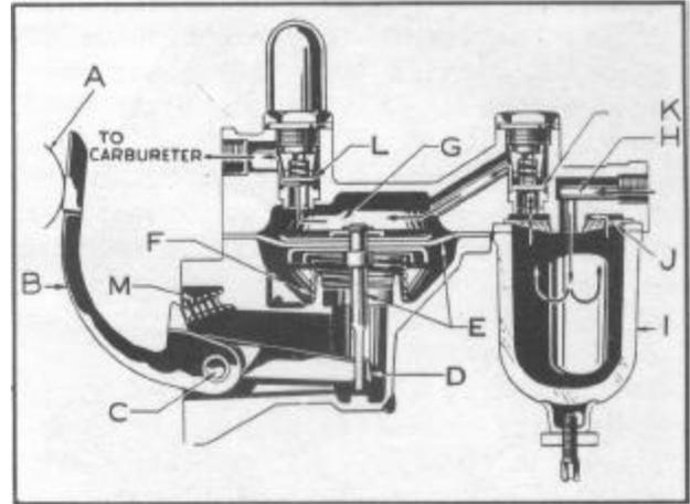
termined by an adjustable drive spring. Delivery pressure with the electric type pump ranges from 2-1/2 to 3 pounds and from 3 to 4 pounds with the mechanical type unit.
