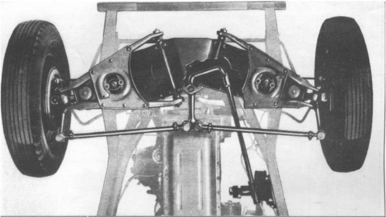
Center Point Steering involves the use of few parts of rugged design including a heavy, adjustable drag link through which the steering effort is transmitted to a steering arm located at the exact center of the chassis. This center steering arm is mounted on a needle roller bearing pivot in the front suspension support frame cross member and transfers the steering movement to each front wheel through two tie rods of equal length.
