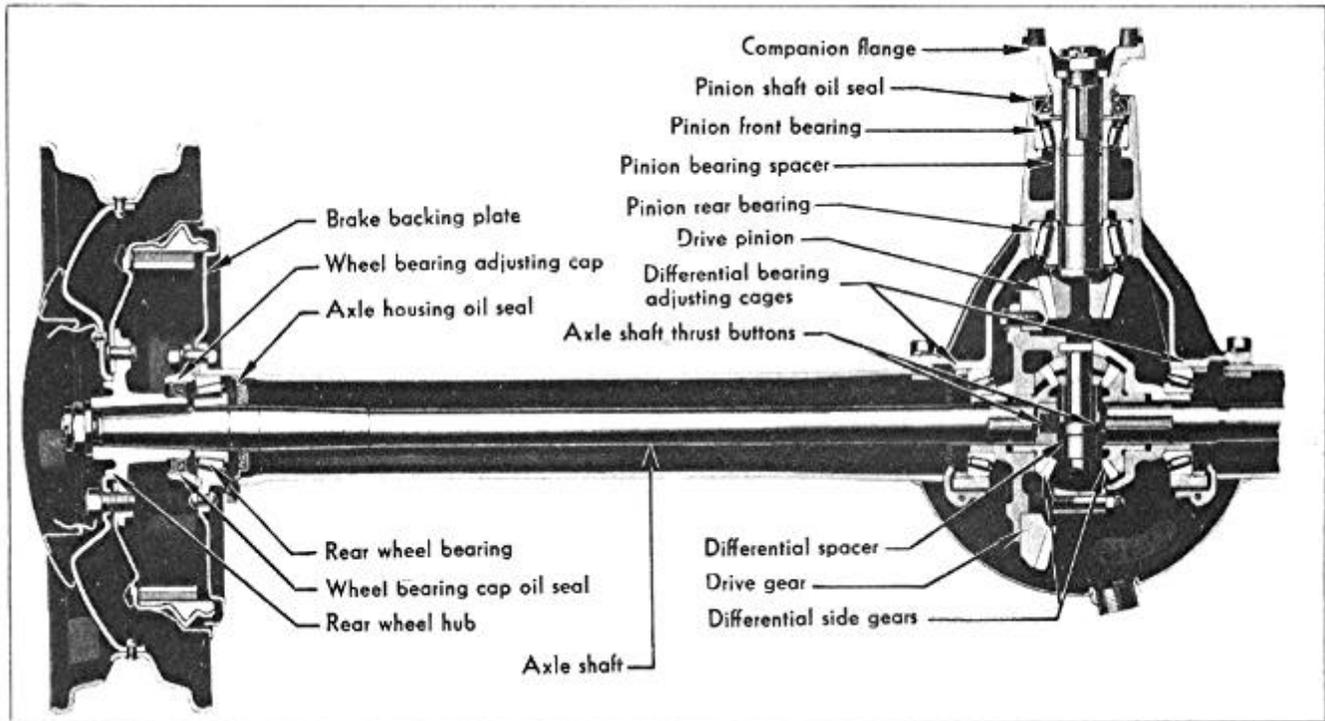
steels are used for all gears and shafts and the drive gear and pinion are of the helical bevel type. Eight bolts are used to attach the drive gear to the flange of the two piece differential case.
