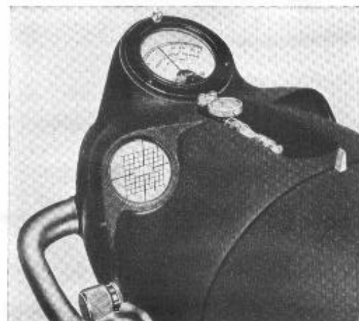
5. The internal screen shows the pattern of the beam against a graduated cross-grid ruling, and enables the customer to see the setting of his lights.
