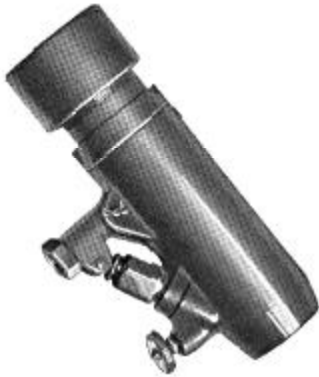
Hydraulic Body Jack—Capacity 10,000 lbs., designed especially for Body work, 6 1/4" stroke and weighing only 12 3/4 lbs.
