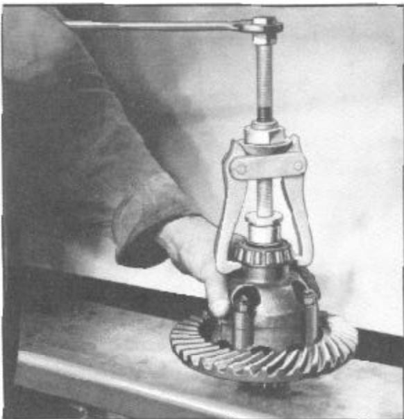
Figure 12--Removing Differential Bearing Cone and Roller
