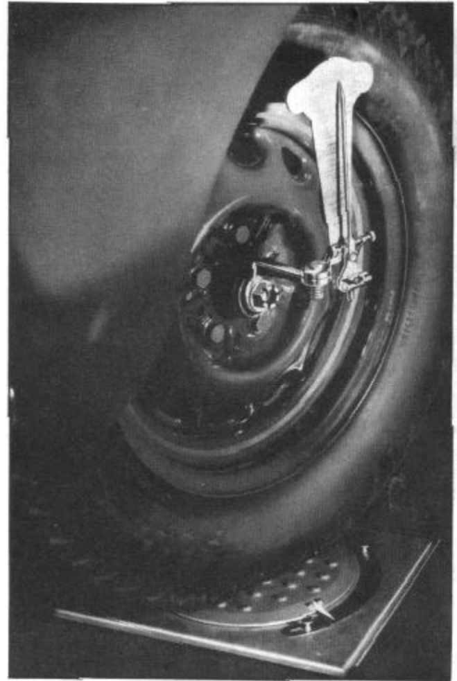
Figure 3--Jiffy Gauge-Checking Caster-First Position
