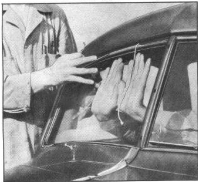
Figure 9--Installing Windshield Glass
