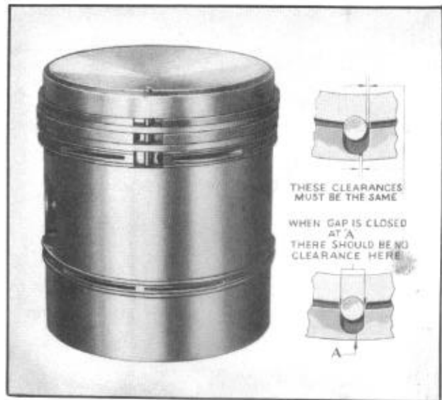
Figure 16--Piston Ring Clearances
