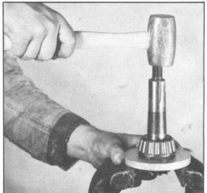
Figure 9--Removing Rear Pinion Shaft Bearing
