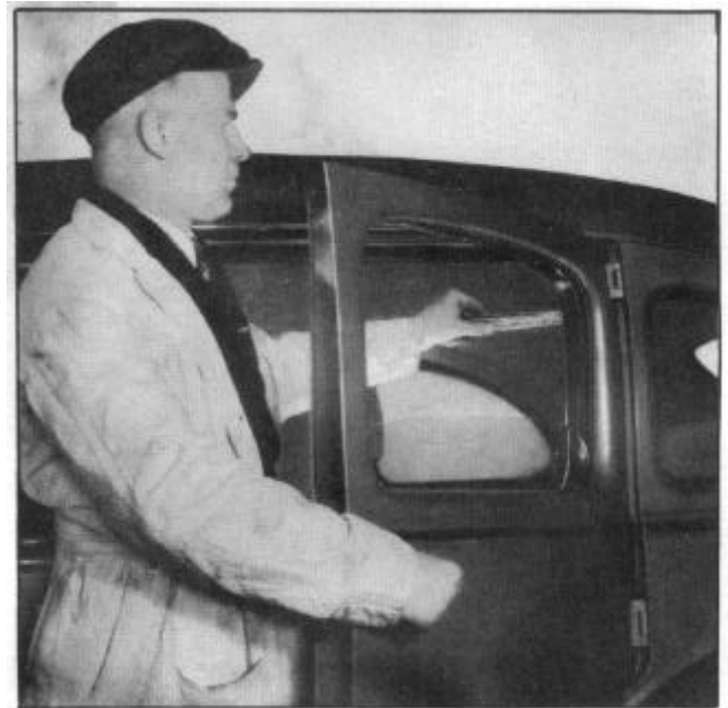
Figure 11--Spreading Door Hinge
