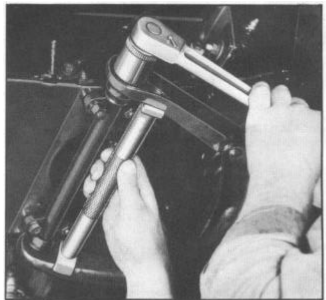
Figure 9--Maintaining Lower Support Alignment Using Tool J 1052
