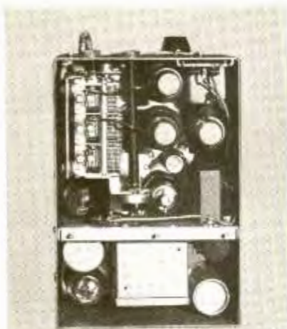
This view shows the 6-tube Superheterodyne chassis with Automatic Volume Control, single Pentode Power-stage, plug-in Vibrator, Tone Control and Noise Filter. Tuning range: 540-1600 kcs.
