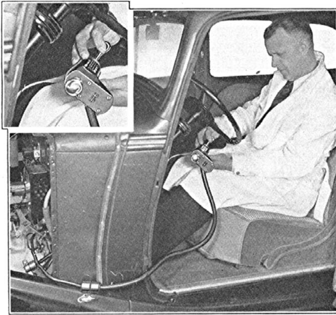
Figure 7 Using Master Selector Switch to make comparative check of Selector Switch and testing for "shorts"
