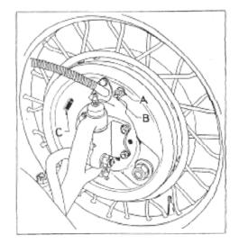
It is necessary to have the brakes adjusted to offset normal wear when the brake pedal can be depressed within  $1\frac{1}{2}$ " of the floor. This adjustment is made as follows:
