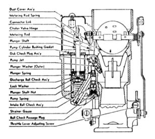
ACCELERATING PUMP: - Low pressure type positively actuated by throttle lever. Fuel drawn into pump chamber through intake ball check valve and strainer on upstroke of plunger and discharged through outlet disc check valve to pump jet in carburetor wall on downstroke of plunger when throttle opened.
