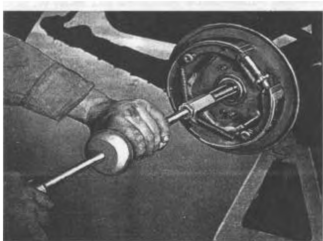
Figure 1307—Removing Axle Shaft and Wheel Bearing—J-352 Axle Shaft and Bearing Puller
