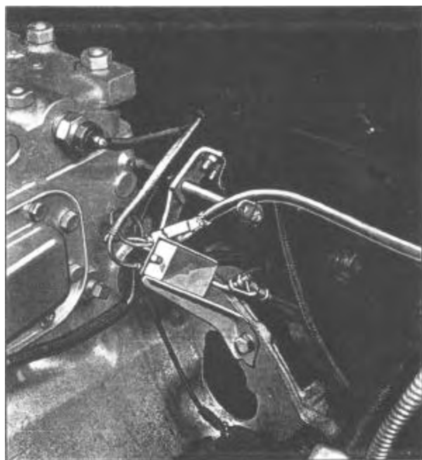
Figure 1116 Connection of test cable to clutch circuit breaker
