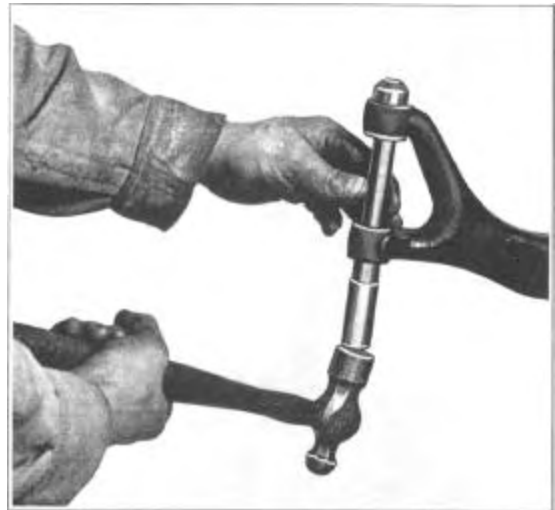
Figure 1508—Installing Pivot Pin Upper Bushing—Tools J-469-2, J-990-2
