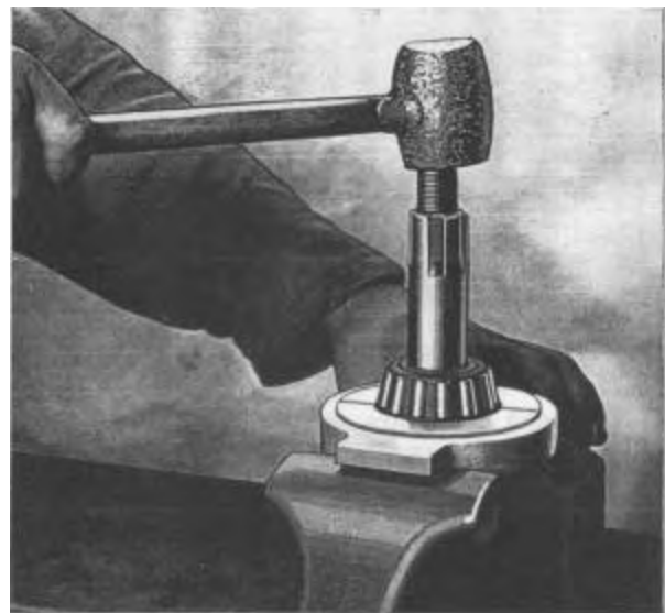
Figure 1311—Removing Rear Pinion Shaft Bearing—J-358 Pinion Shaft Bearing Remover
