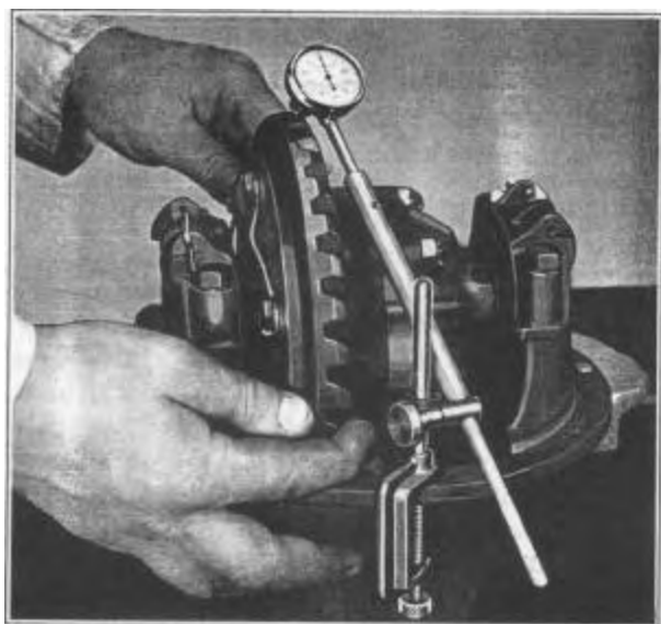
Figure J1318—Checking Drive Gear and Pinion Backlash— J-390-X Dial Indicator
