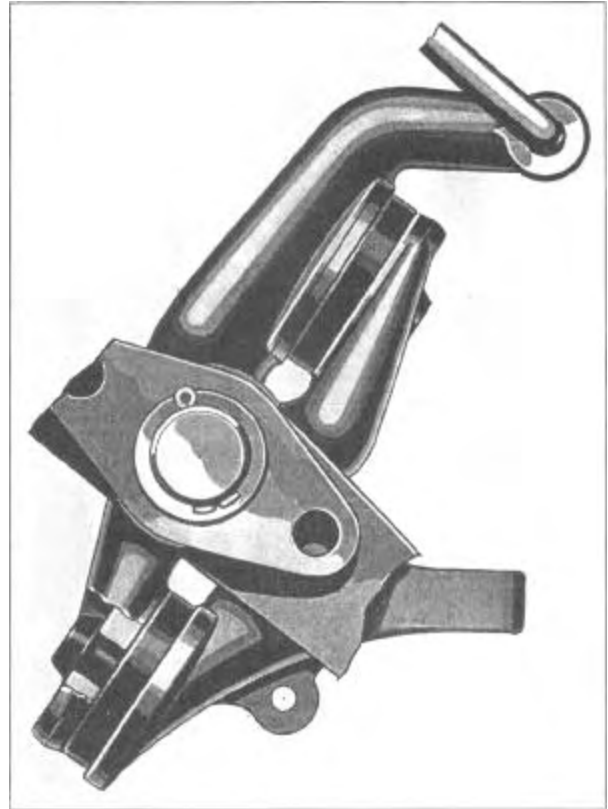
Figure 803—Details of 1937 Clutch Linkage Rubber Pads
