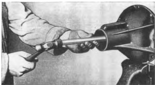
Figure 1313—Removing Front and Rear Pinion Shaft Oil Bearing Caps—HM-63 Pinion Bearing Cup Remover
