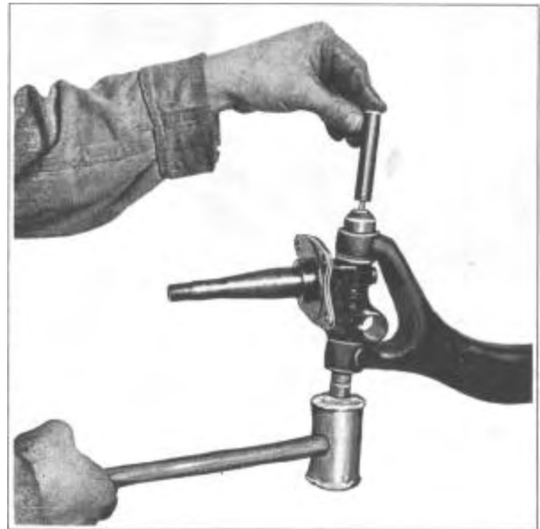
Figure 1512—Installing Pivot Pin—Tool J-479-1 used as guide
