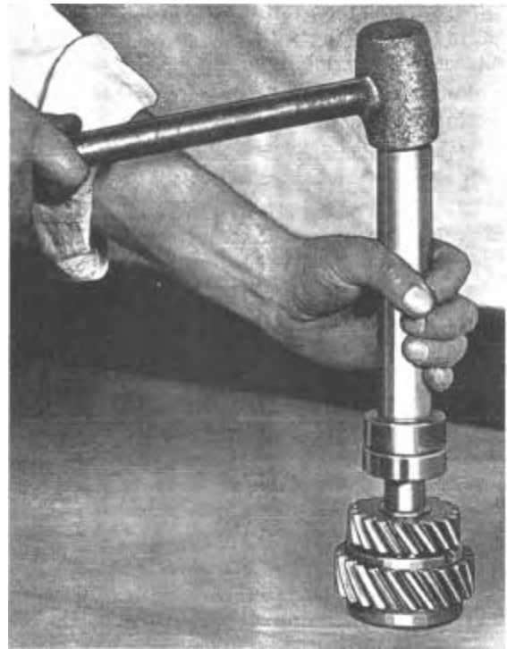
Figure 1014—Installing Main Drive Gear Ball Bearing— J-779 Bearing Installing Tool
