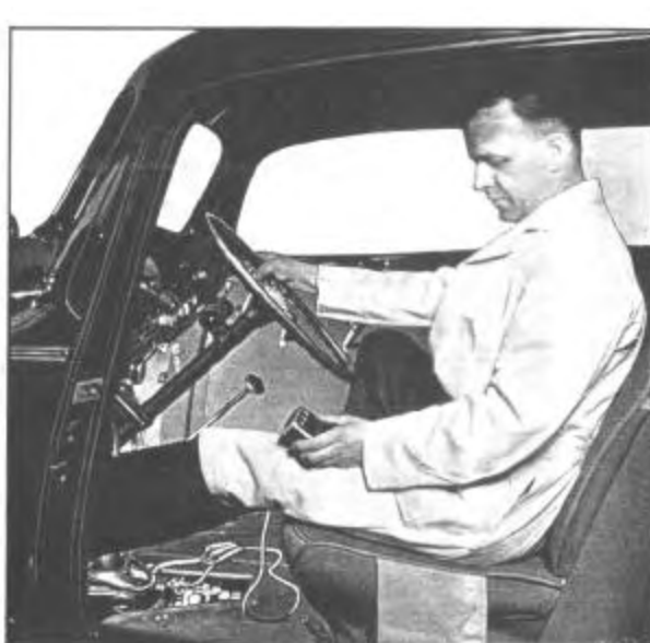
Figure 1115 Testing circuits in lower harness and switches Insert shows connection of test lamps to lower harness
