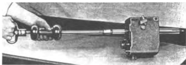
Figure 1004—Removing Mainshaft and Rear Bearing— J-352 Shaft Puller, J-778 Adapter
