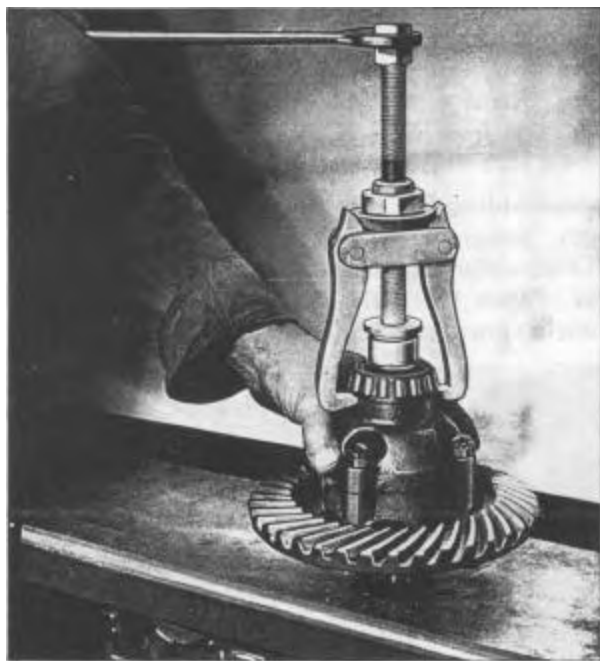
Figure 1314—Removing Differential Bearing Cones and Rolls—J-354 Bearing Puller
