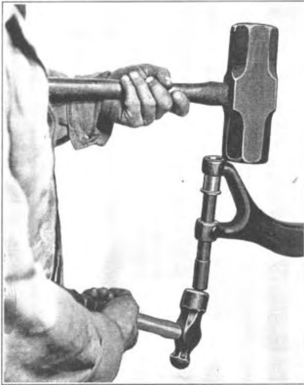
Figure 1508—Installing Pivot Pin Upper Bushing—Tools J-469-2, J-990-2
