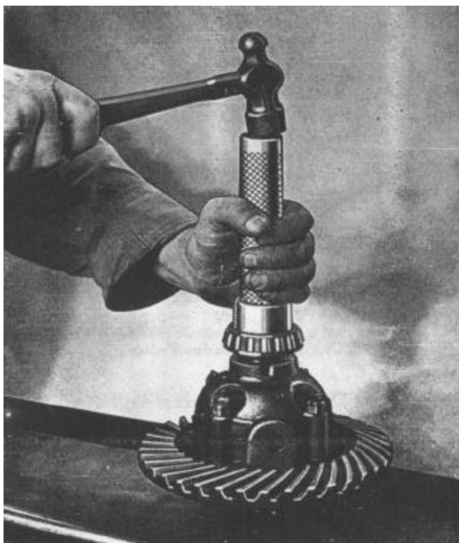
Figure 1315—Installing Differential Bearing Cones and Rolls—J-355 Differential Bearing Driver
