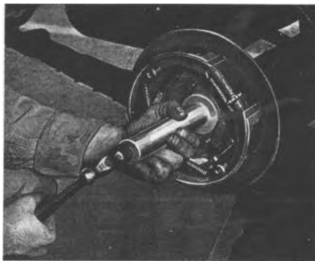
Figure 1319—Installing Axle Shaft Oil Seal Assemblies— J-353-2 Oil Seal Replacer
