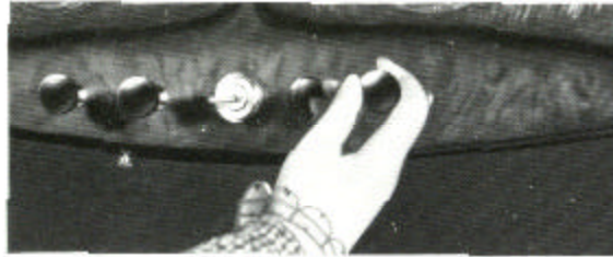
The handy Ride Control on the dash makes available the widest possible range of shock absorber action.
