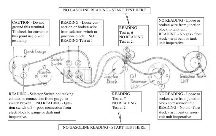
It is advisable to test individual units after removal from the car and before installation. Although a test for operation of the dash unit can be made by connecting it direct to a battery (should show full) it is advisable to connect a tank or reservoir unit in series so that the gauge reading can be varied and the operation watched.
