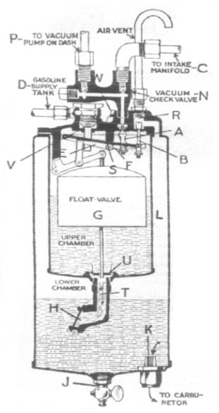
A is the suction valve for opening and closing the connection to manifold and through which a vacuum is extend from the engine manifold to gasoline tank.
