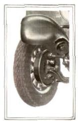
Internal expanding Bendix fourwheel brakes are protected from dirt, self-energizing
