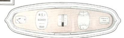
The decorative instrument panel, indirectly lighted, includes a gasoline gauge and motor heat indicator
