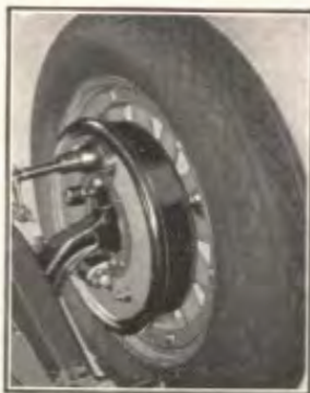
Hudson's four-wheel brakes are of the self-energizing type. Action is smooth, sure and un-failing.
