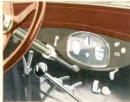
On the instrument panel such equipment as a gasoline gauge, electrolock, carburetor choke, manifold heat control and radiator shutter lever give the Hudson driver centralized car control
