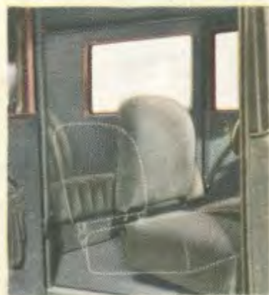
The right front seat slides forward—whether vacant or occupied—so that passengers may reach the rear seats with entire ease. This seat arrangement is new and is exclusive to Hudson-Essex
