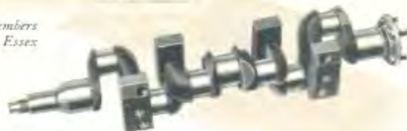
The patented Super-Six design of the Essex crankshaft produces a perfect flywheel type of balance, preventing engine vibration before it happens
