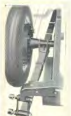
Alloy steel semi-elliptic springs, special at their rear ends, give riding comfort and prevent unpleasant sideway
