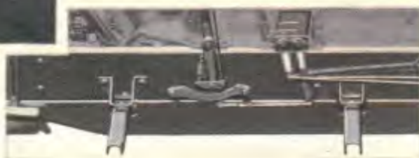
The effective depth of the Essex frame side members is 8 inches, a solid foundation for sturdy Essex bodies
