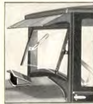
A cowl ventilator is a distinct advantage
