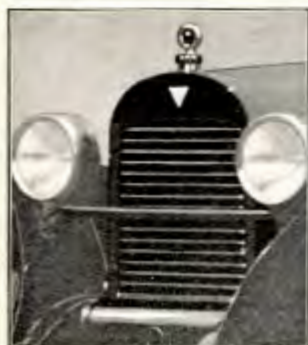
With motormeter and shutters you can regulate the running heat of your motor
