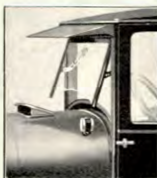
A cowl ventilator is a distinct advantage
