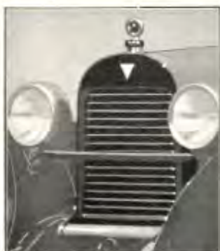
With motometer and shutters you can regulate the running heat of your motor
