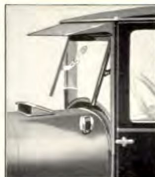
A cowl ventilator is a distinct advantage
