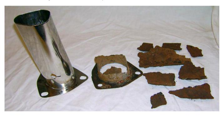
Included with this bulletin is a detailed measured drawing provided by John Meadows of Victoria, Australia. He created this drawing using an original NOS Essex 4 Water Inlet Deflector. I used this drawing, & measurements to fabricate the stainless steel replacement you see in the above picture, and am successfully running in my car today.
